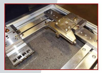
Stainless steel precision ground tooling system eliminates the need for additional tooling needs, while standard 25mm hole spacing allows for compatibility user's existing tooling brands.
