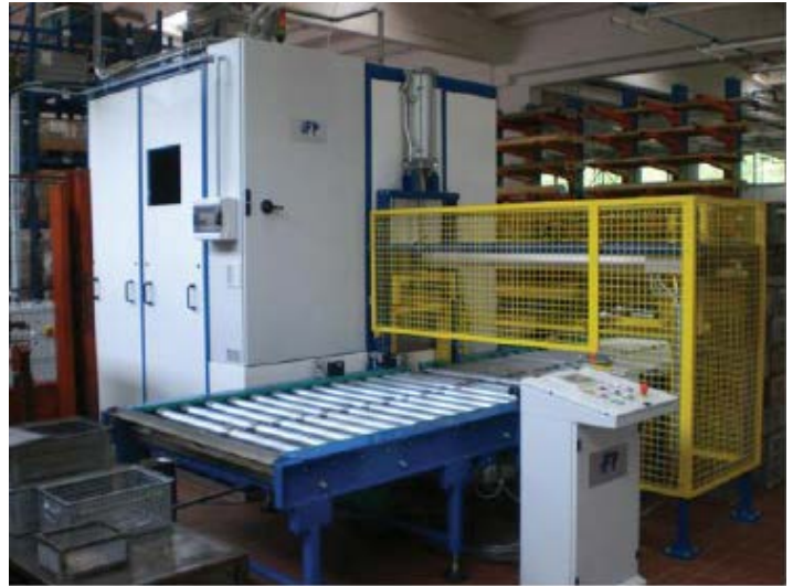
iFP Kleen Power vacuum parts washer with optional automation system
