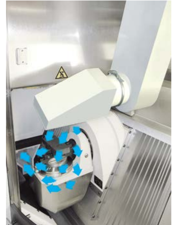
Graphite extraction using a powerful suction system
