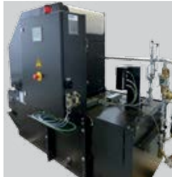
Cooling lubricant filtration
